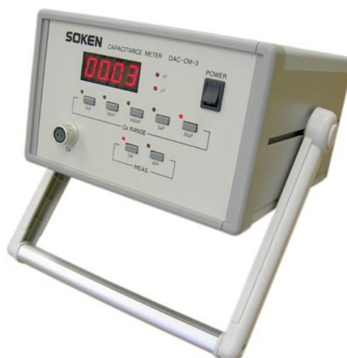
Model DAC-CM-3 is a Capacitance Meter for testing Capacitance of Electrical Instruments which gave thoroughgoing protective measures to induced voltage or residual voltage. Since a testing power supply of enough Capacity AC100V is built in, the error caused by induced voltage is suppressed to the minimum. DAC-CM-3 enables reliable and repeatable measurement of specimen like power cables, etc.
