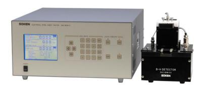
DAC-BHW-5 is AC Magnetic Core Loss Tester for Single sheet (Single Strip Tester) to test electromagnetic steel sheets. Introducing Magnetic Potentiometer Method, influence by air gaps between test specimen and detector is minimized. B-H Curve can be observed by connecting an oscilloscope. Different testing coils (D1, D2, and an optional D3) are provided for wide measuring range.
