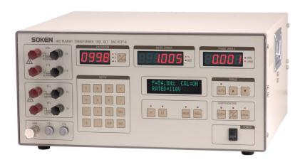
DAC-VCTT-8 is a device designed for quality testing of instrument current and voltage transformers. It can measure the ratio error and phase angle of instrument transformers in accordance with the international standards.
